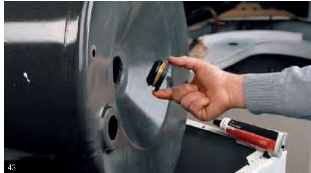
In washing machine repair, 3M™ Neoprene High Performance Rubber and Gasket Adhesive 1300 bonds with high immediate strength and seals the doughnut ring seal in the outer tub.
